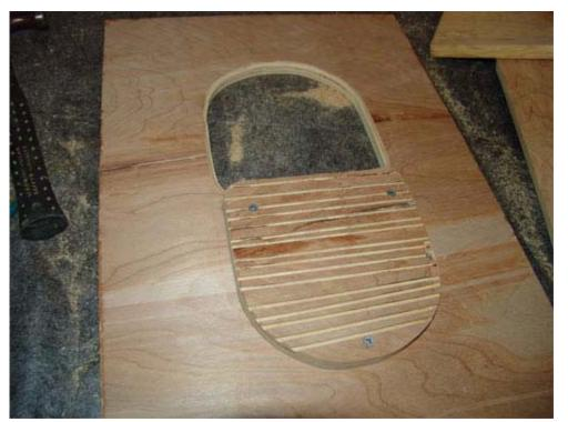
If you made the notches with a radial arm saw, table saw, or router, then screw the latter into place with 3 screws (1-1/4 to 1-1/2" long).
