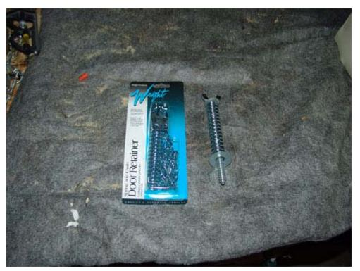
Compression springs are hard to find, so the best ones can be obtained from (2) door retainer kits. Door retainer kits can be purchased from any hardware store.
