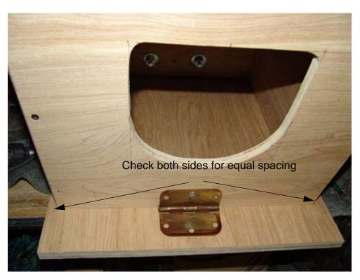
The easiest way to attach the hinge is to turn the owl house upside down. Place the hinge in the middle.
